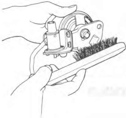
Fig. EC-36 Cleaning E.G.R. control valve seat
