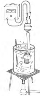
Fig. EC-39 Checking water temperature switch operation
